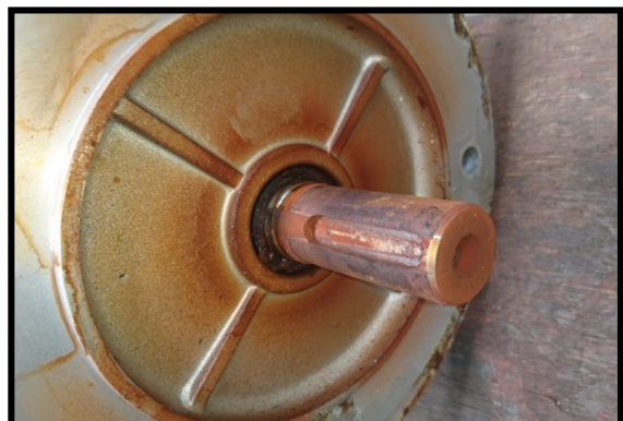
Fig. 6. Shaft Motor and keyway with wear
